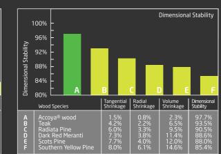
N.B. This graph shows the dimensional stability (volume metric) from fully soaked to oven dry (the most extreme laboratory test). Where a material is unaffected by moisture changes the dimensional stability would be 100%. This table does not show changes due to temperature conditions (wood is very stable). The main table on the previous page shows the shrinkage in more normal weather conditions (with simulated humidity varying between
